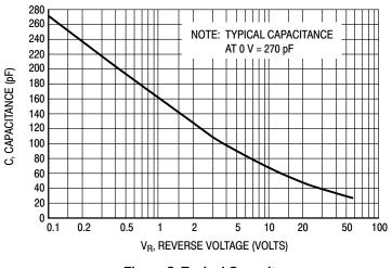
Figure 5. Typical Capacitance
