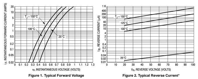
\*The curves shown are typical for the highest voltage device in the voltage grouping. Typical reverse current for lower voltage selections can be estimated from these curves if V<sub>R</sub> is sufficient below rated V<sub>R</sub>.
